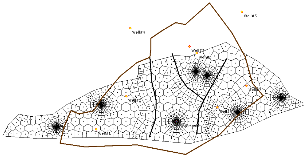
Fig. 10.E.9 – Equivalent Voronoi grid for an anisotropic reservoir ( k_x/k_y=0.2 )
