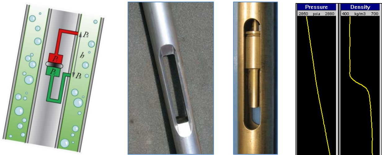
Fig. 14.C.5 – Schematic of a gradiomanometer; nuclear density tool; TFD tool; pressure differentiation
