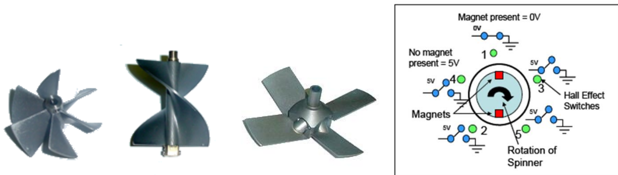
Fig. 14.C.2 – Various types of spinners – Schematic of the Hall effect – Courtesy Sondex
